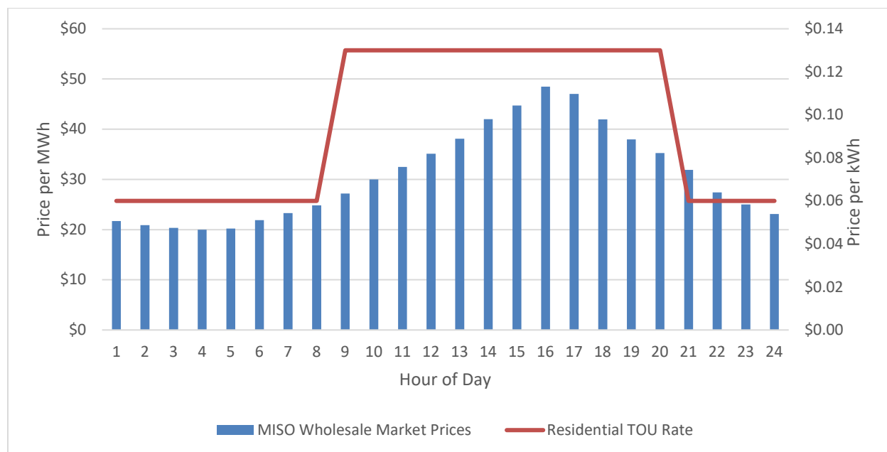
Figure 4-9 Time Varying Price of Electricity on an Average Summer Day in Wisconsin
