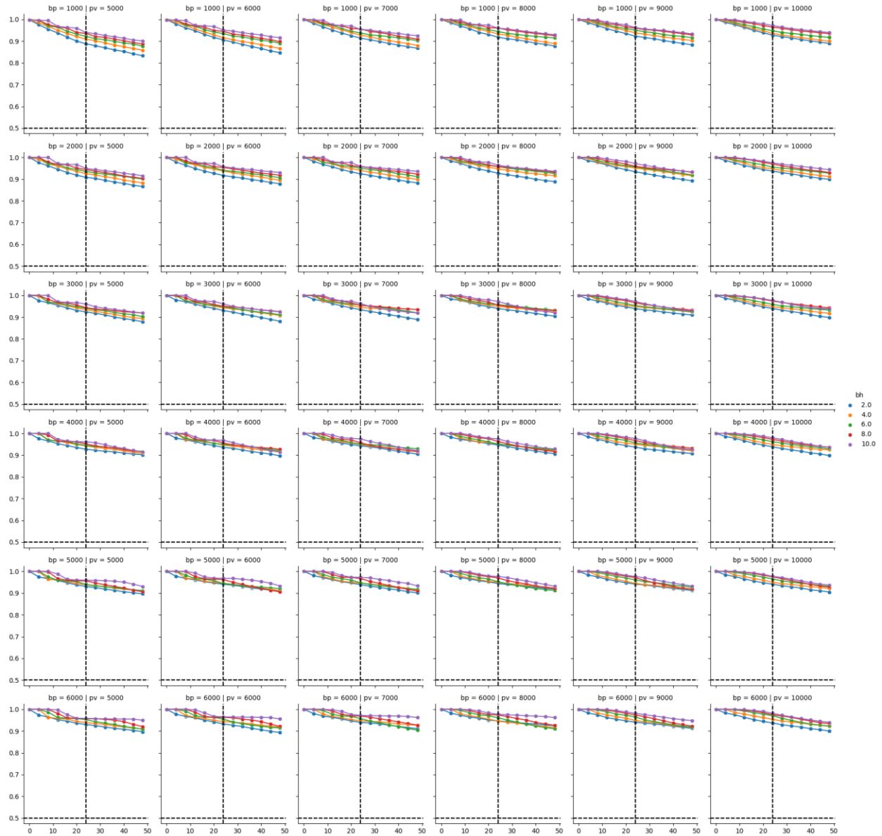
Figure 19 - Resilience performance modeling for total generator capacity of 5 MW (2.7 MW of existing included)
