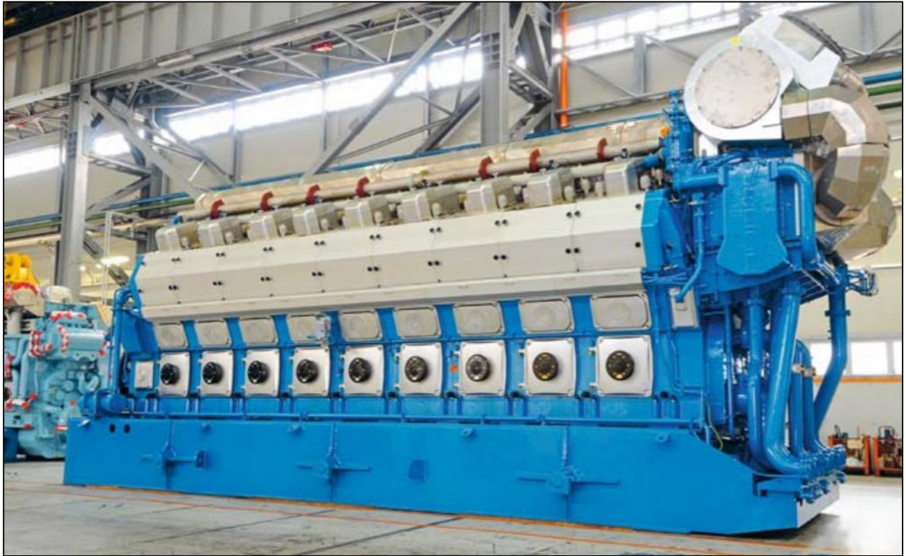
Figure 2-1 An example of a Wärtsilä RICE engine similar to the ones proposed (photo from Wärtsilä trade publication)
