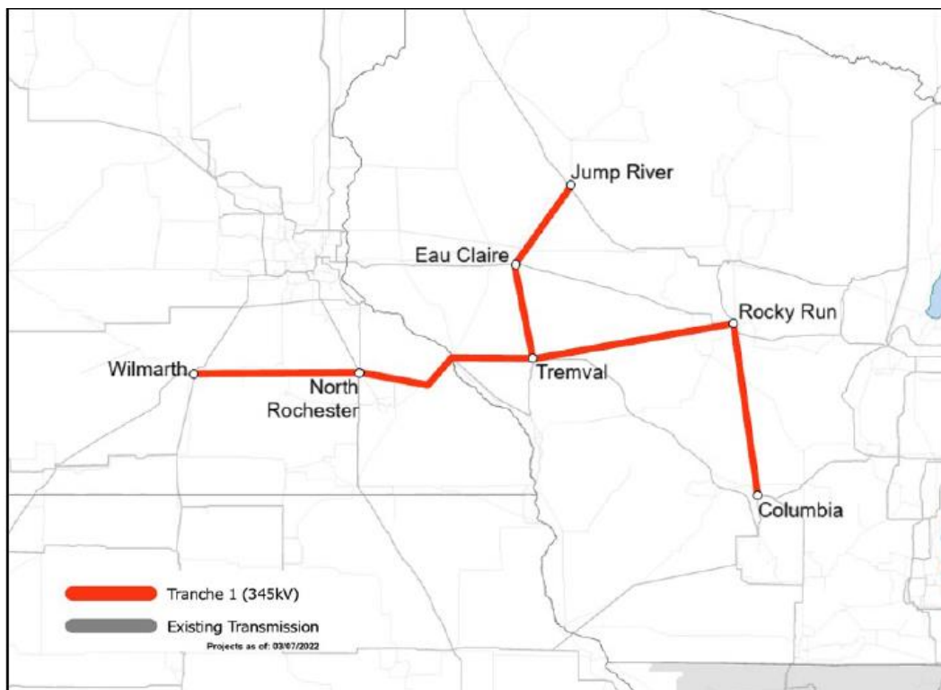
Figure 4-7 LRTP Tranche 1 Transmission Projects in Wisconsin
